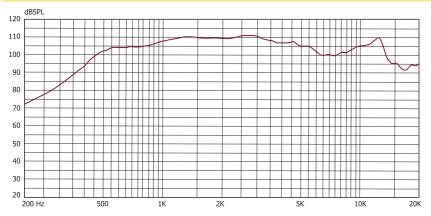
Frequency (Hz), Measured-1W@1M
